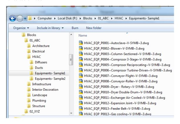
In the image option, user needs to set up the file name of the image (block name, description, layer and color number) and corresponding drawing file should accompany with only block name as shown below.
