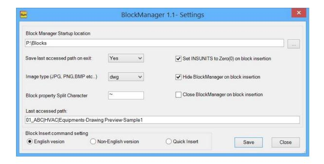
**Save last accessed path on exit:** Set to "Yes" saves the last accessed directory and loads files and images from the saved location during the application startup and Set to "No" loads files and images from the first directory in the list
